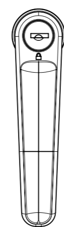
WW = 72 STAINLESS STEEL SCALP AND SHUTTER, KEY LOCKING, REVERSIBLE KEY CODE R001
