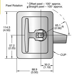
Adjustable-grip Turn handle 90° to latch/unlatch. Additional turns to pull up tighter, compress a gasket.
