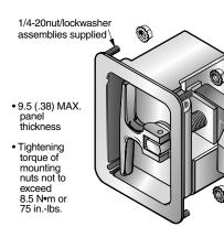
Loosen jam nuts to adjust pawl to exact grip. Tighten jam nuts to lock pawl in position.
