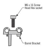
Pulley Bracket Sub-Assembly
