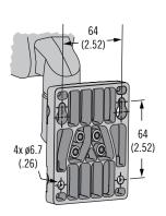
Wall Mount, Rear Fastened K=0(1.50)38 4x M5 x 0.8 (1.81)**Optional** wire notch K=1
